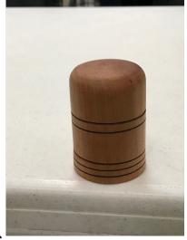
waste piece was then trimmed down to use as a jam chuck so the bottom of the box could be cleaned up with a skew. When shaping the bottom he made it concave so that it would sit flat.
