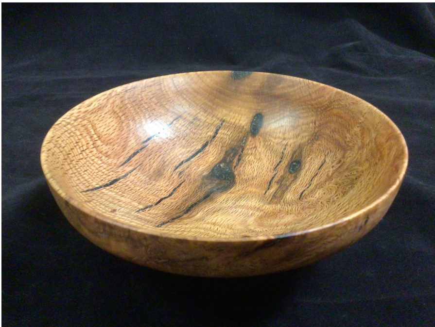
Terry Butler—This “OTF—Off the Floor” wood had cracks that had to be filled with coffee grounds and CA glue. The finish is Howard Wax.
