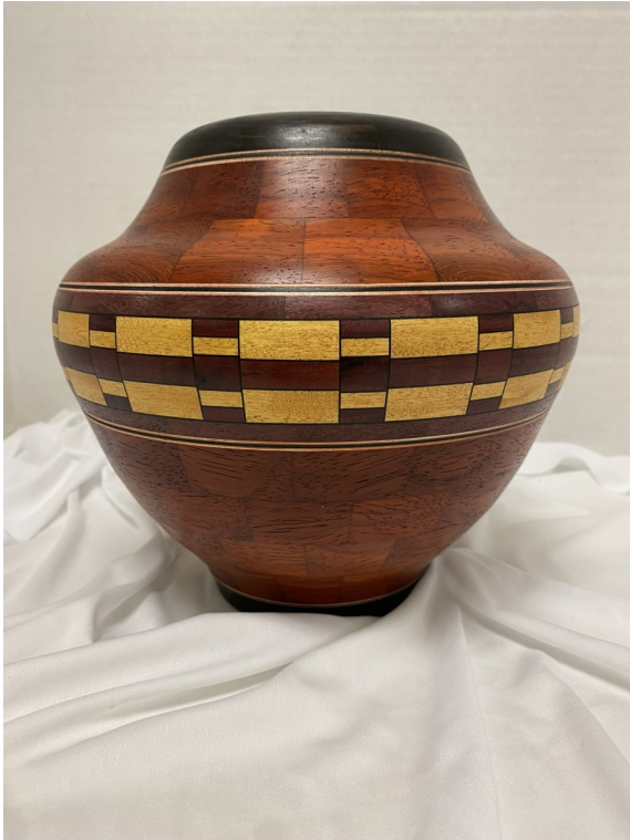
Joe Meskaitis—Segmented vase made from Padauk, Yellow and Purple Heart. Finish is Sanding Sealer and wipe on Poly.
