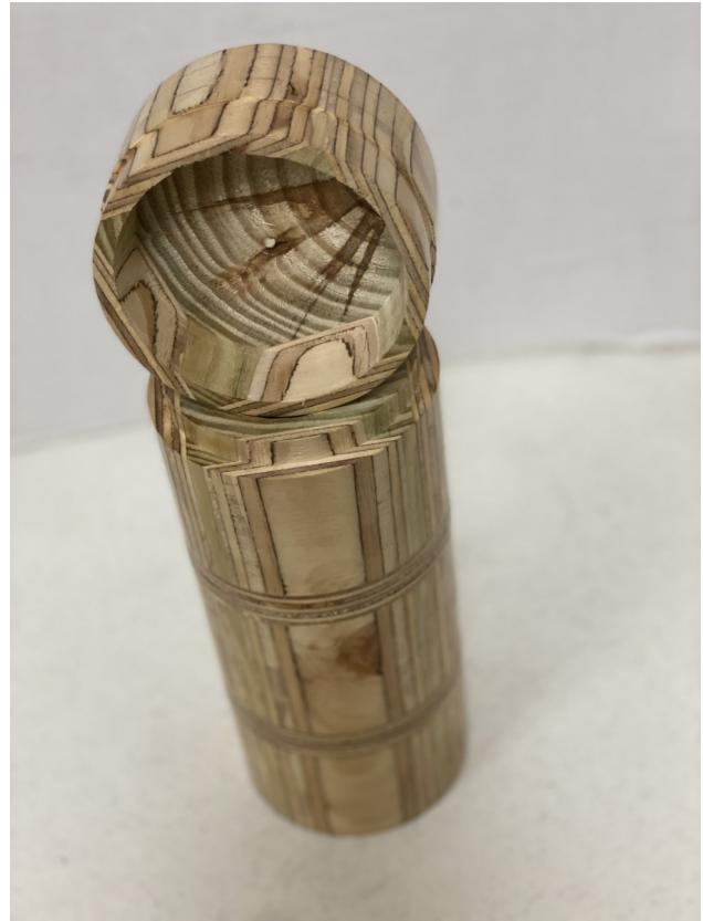
Bernie Martinson—Plywood fireplace match box. Finish is sanding sealer and six coats of spray on poly.
