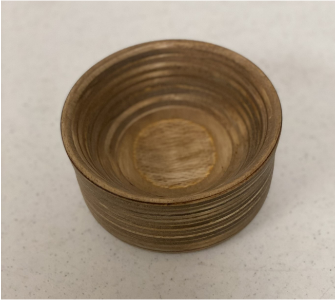
Jeff Fairchild—Potpourri bowl made from Maple plywood. Finish is oil based MIN-WAX.
